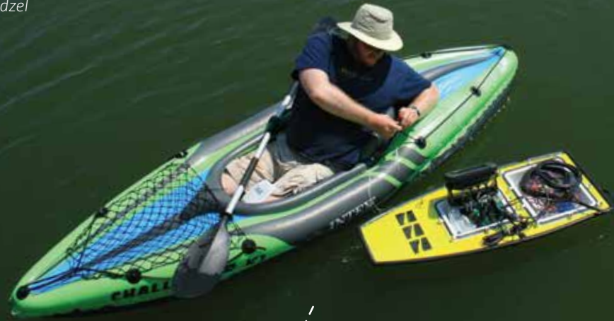
Graduate student Thane Somers services a robotic surface vehicle. The boat pictured does not travel under water like a torpedo-shaped AUV used in field trials, but it was used to test Geoff Hollinger's algorithm designed to train AUVs to learn human preferences.
