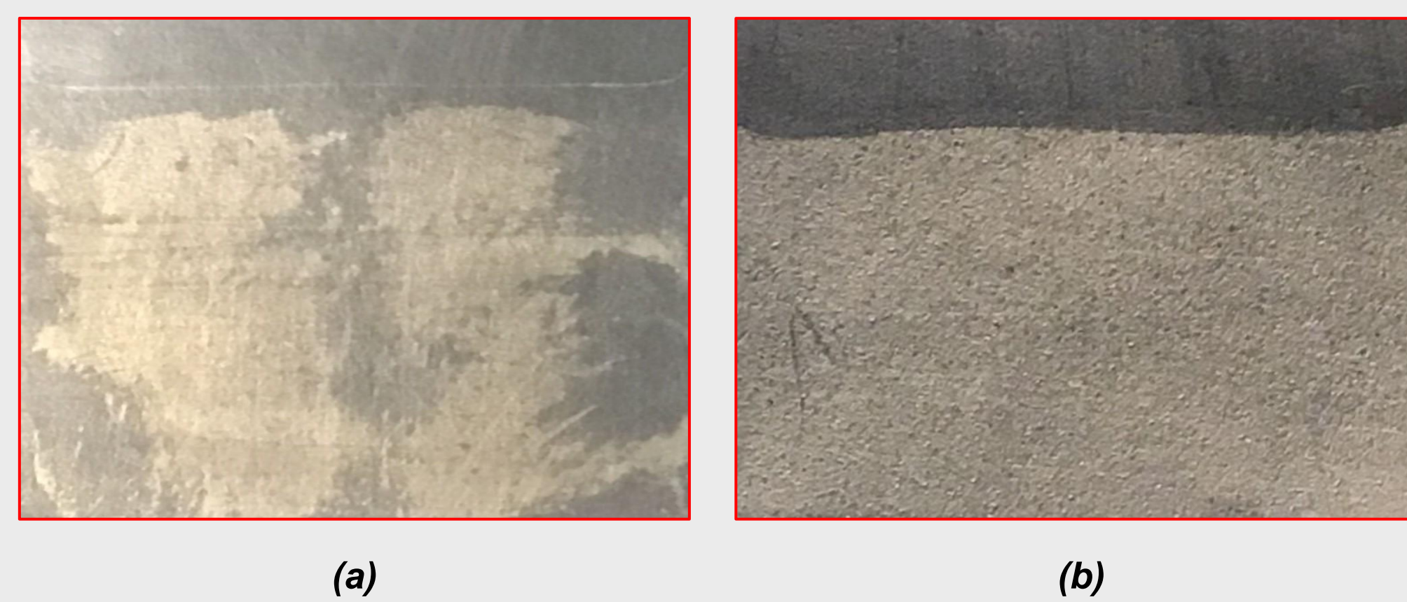
Figure 5. Examples of nickel plating with and without the elimination of side reactions. The silver is the nickel and the gray is the graphite. (a) Sample with deposited nickel where side reactions are also occurring, (b) Sample with deposited nickel where the side reactions have been eliminated
