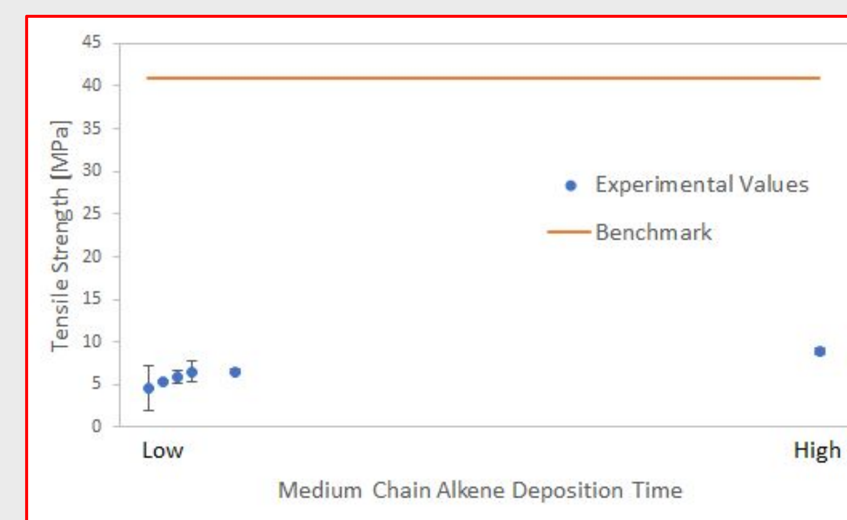
Figure 9. The figure above depicts the tensile strength measurements of alkene-impregnated bipolar plates in relation to the deposition time of the medium chain alkene. Error bars represent standard deviation and experimental data is compared to the tensile strength benchmark of a standard industry bipolar plate. Samples tested were cut into dog-bone geometry and measured with Instron 5969.
