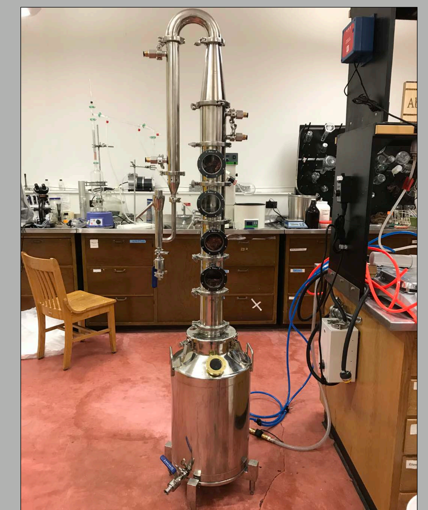
Figure 7: Distillation column as set up in lab. Is used for demonstrations and graduate research.
