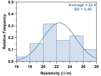
Data shown is from a central mix plant with one mixture run frequently, low variation Spragg et al. 2012
