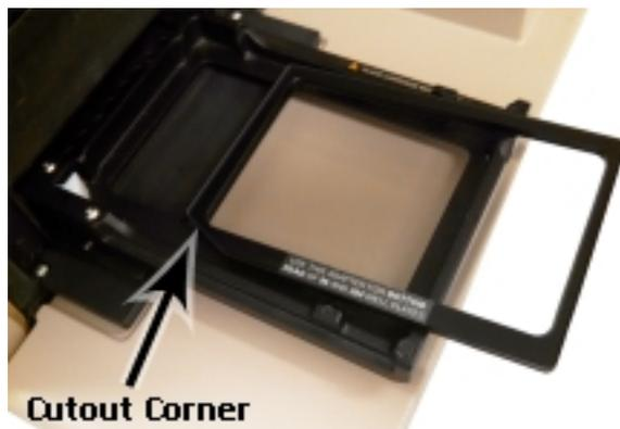
4. For 6-well, 12-well, 24-well, and 48-well plates, remove the black plate adapter.
