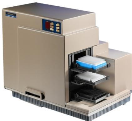
The instrument's dual monochromators enable you to target the optimal assay excitation and emission wavelengths and eliminate the need to change expensive band pass filters between experiments. The two holographic diffraction grating monochromators enable you to select any wavelength in the following ranges:
