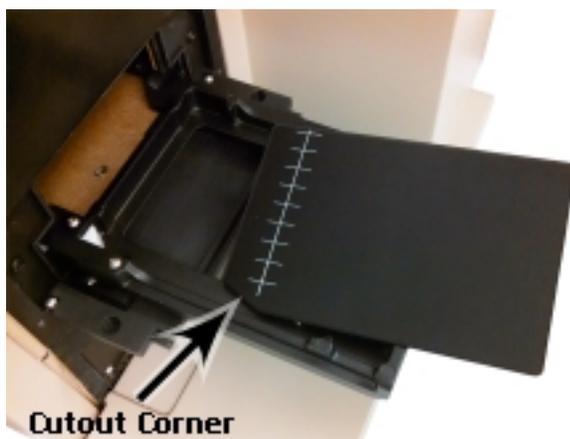
4. Insert the filled compound plate into the drawer, with well A1 in the upper left corner of the drawer. Make sure the compound plate is flat against the compound baseplate.
