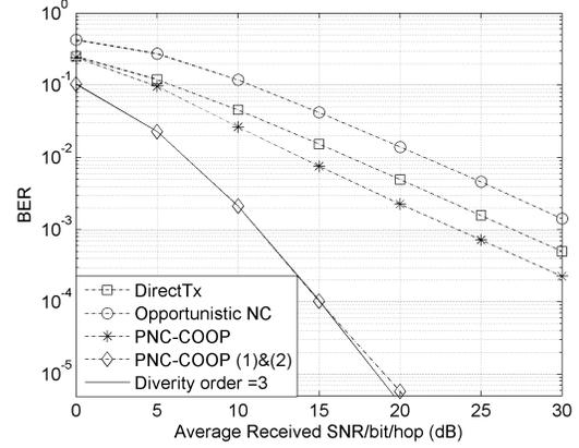
Figure 6. Average end-to-end BER when the network encode amount  $k=3$
