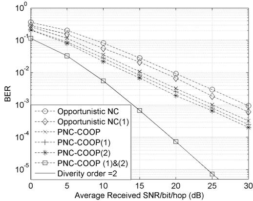
Figure 5. Average end-to-end BER of the network shown in Fig. 1 with different conditions
