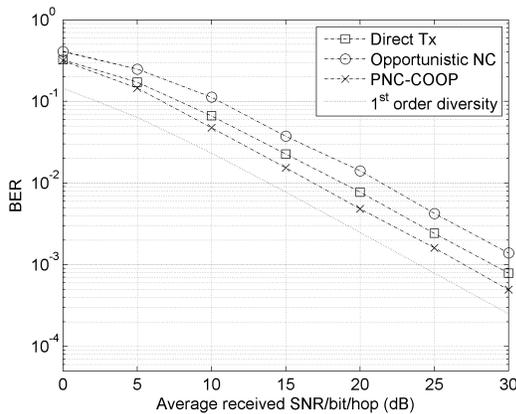
Figure 7. Average end-to-end BER over a 16 nodes wireless ad hoc network using setting described in section III.B
