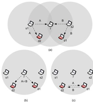
Figure 1. Example of PNC-COOP strategy: (a) Node  $s_1$  sends data  $A$  to  $d_1$  and node  $s_2$  sends data  $B$  to  $d_2$  via node  $r$ . (b) Node  $r$  overhears and relays  $A \oplus B$  to  $d_1$  and  $d_2$ . (c)  $d_1$  and  $d_2$  cooperate to be a partner of one another and forward the data that each needs
