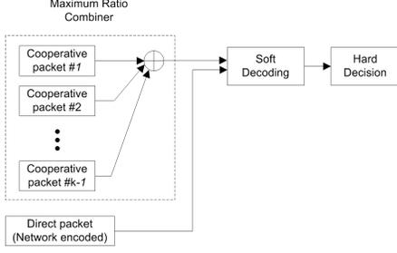
Figure 3. Decoder for PNC-COOP
