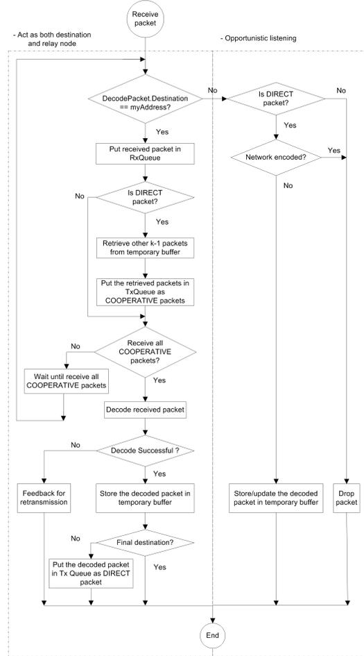
Figure 2. Link layer design for the PNC-COOP receiver
