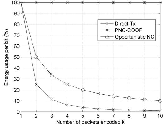
Figure 10. Transmitted energy per information bit at the sender node for different amounts of network coding
