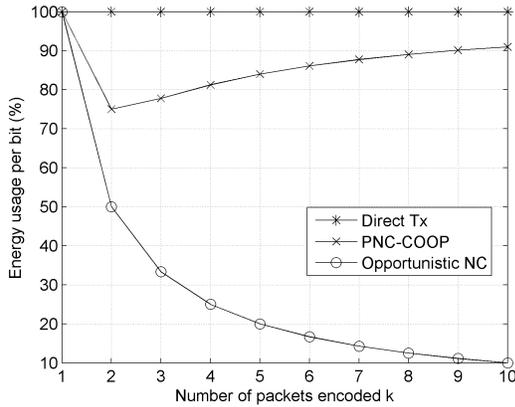
Figure 9. Transmitted energy per information bit for different amounts of network coding
