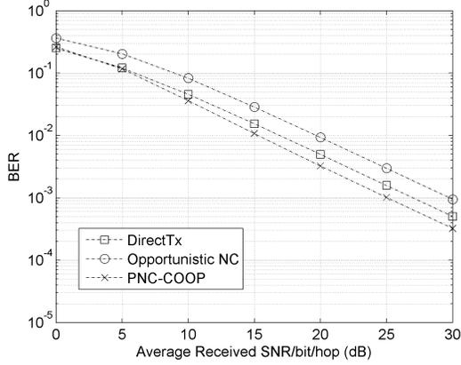
Figure 4. Average end-to-end BER of the network shown in Fig. 1 when the network encode amount  $k=2$
