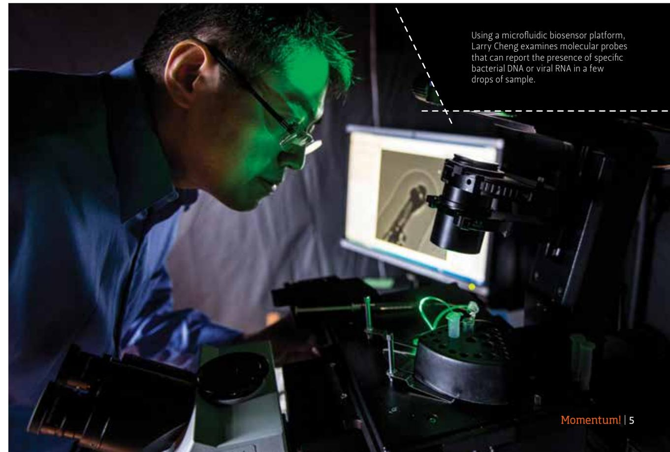
Using a microfluidic biosensor platform, Larry Cheng examines molecular probes that can report the presence of specific bacterial DNA or viral RNA in a few drops of sample.
