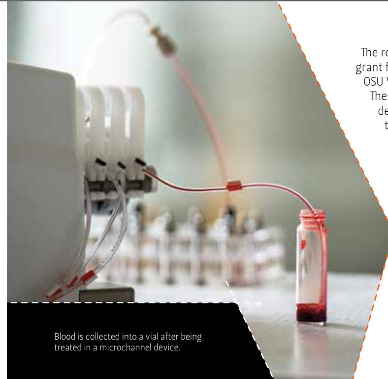
Blood is collected into a vial after being treated in a microchannel device.
