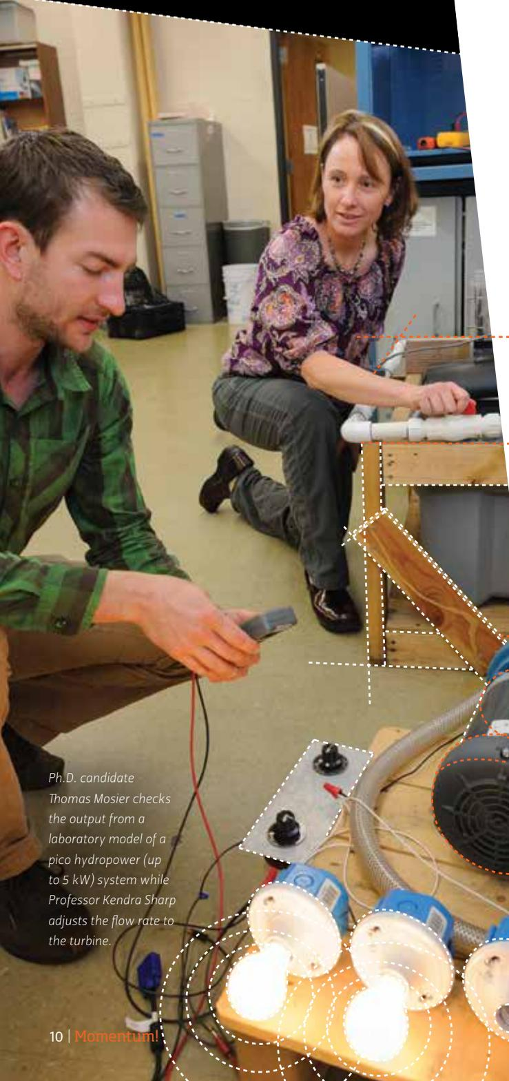
Ph.D. candidate Thomas Mosier checks the output from a laboratory model of a pico hydropower (up to 5 kW) system while Professor Kendra Sharp adjusts the flow rate to the turbine.
