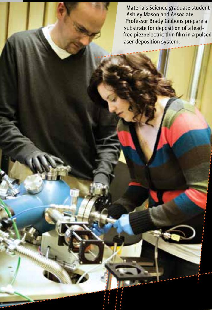
Materials Science graduate student Ashley Mason and Associate Professor Brady Gibbons prepare a substrate for deposition of a lead-free piezoelectric thin film in a pulsed laser deposition system.
