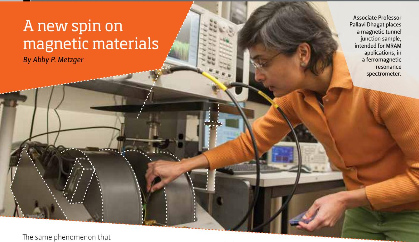
Associate Professor Pallavi Dhagat places a magnetic tunnel junction sample, intended for MRAM applications, in a ferromagnetic resonance spectrometer.
