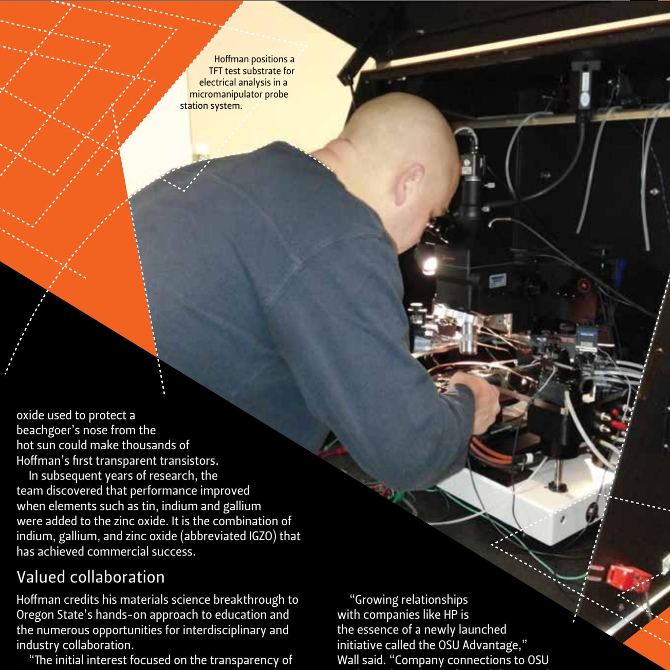
Hoffman positions a TFT test substrate for electrical analysis in a micromanipulator probe station system.
