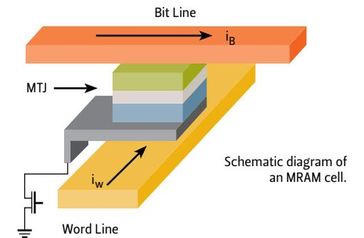
Schematic diagram of an MRAM cell.
